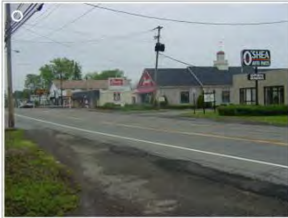
Street with wider vehicle lanes, no curbs allows less restrictive vehicle access.
